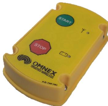
Figure 3.3: The PR2 wireless run-stop.
