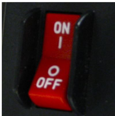
Figure 18.1: The PR2 DC breaker switch in the ON position.
