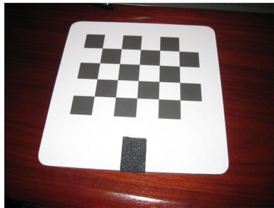
Figure 3.7: Small calibration target.
