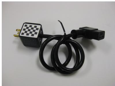
Figure 3.5: The PR2 self plug-in power cord.
