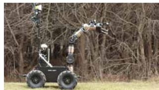
The Husky A200 can easily **interface with** many small industrial **manipulators** for tele-operated or autonomous manipulation tasks.
