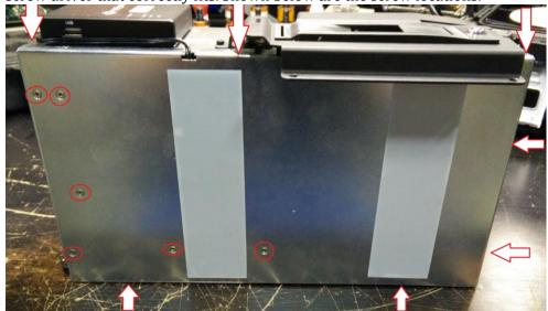
4. Next removing the 2 Phillips screw from the top of the server that fasten the middle tray. Locations shown below.
