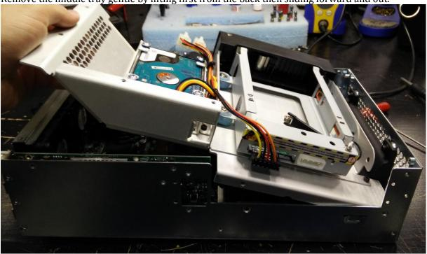
8. Once the middle tray is free the motherboard will be visible. The small coin sized CMOS battery is hiding in the upper left side under cables. Lift the SATA cables out of the way and, if needed, with a pair of small pliers unplug the extra USB cables to gain easy access to the battery
