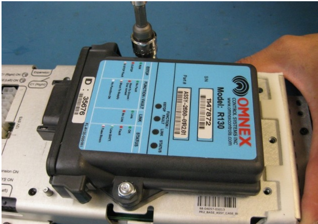
Drawing 17: Remove runstop from power board. Use a grounded work surface.
