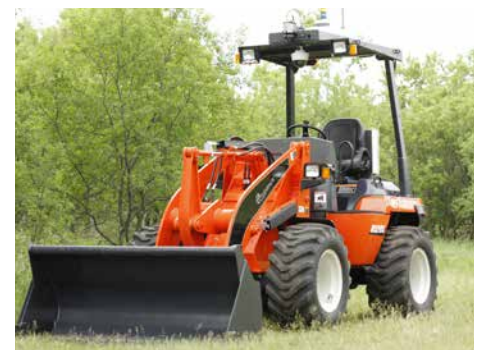
The standard tractor was retrofit into an autonomous loader.
