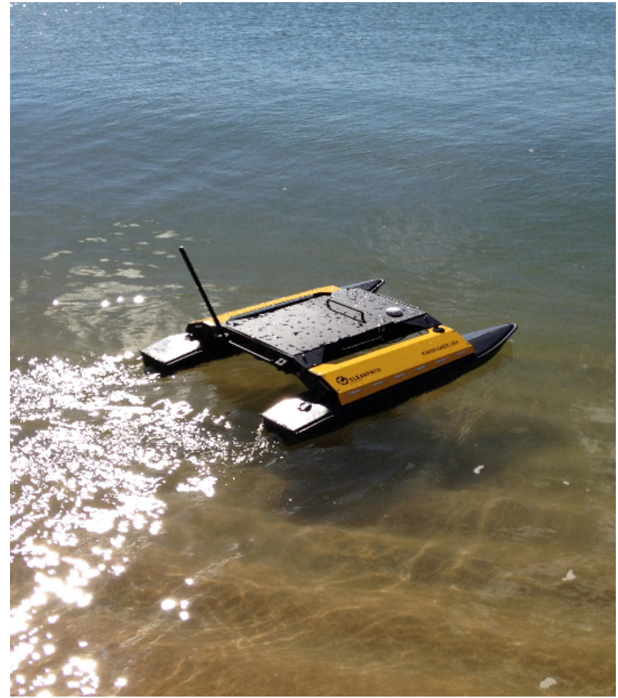
REMOTE SURVEYOR CONFIGURED FOR BATHYMETRIC SURVEY
