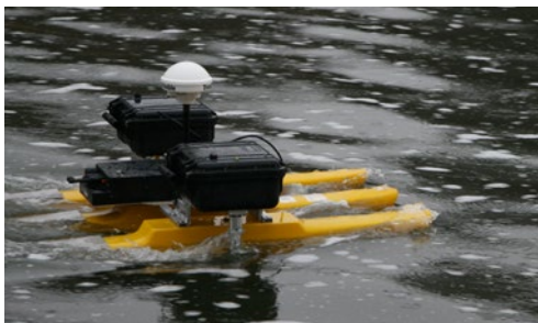
The original Kingfisher Remote Survey System as used by PotashCorp.
